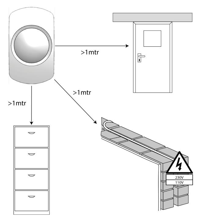
Ensure the devices field of view is not obstructed
